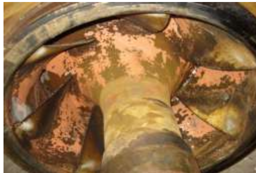
Suction Cavitation marks observed at the eye of the impeller.
