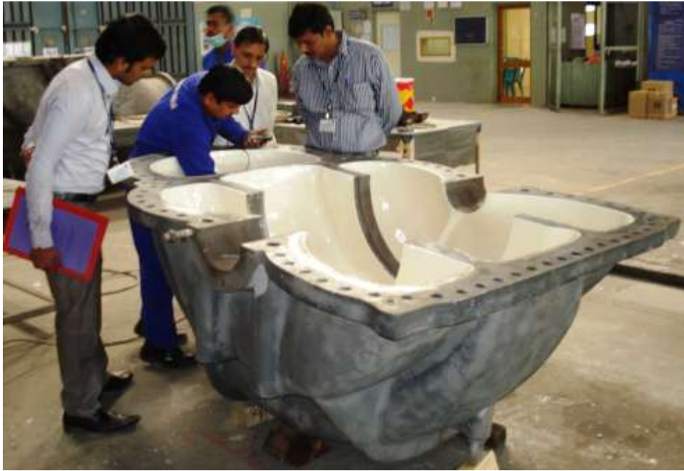
DFT – Thickness measurement
